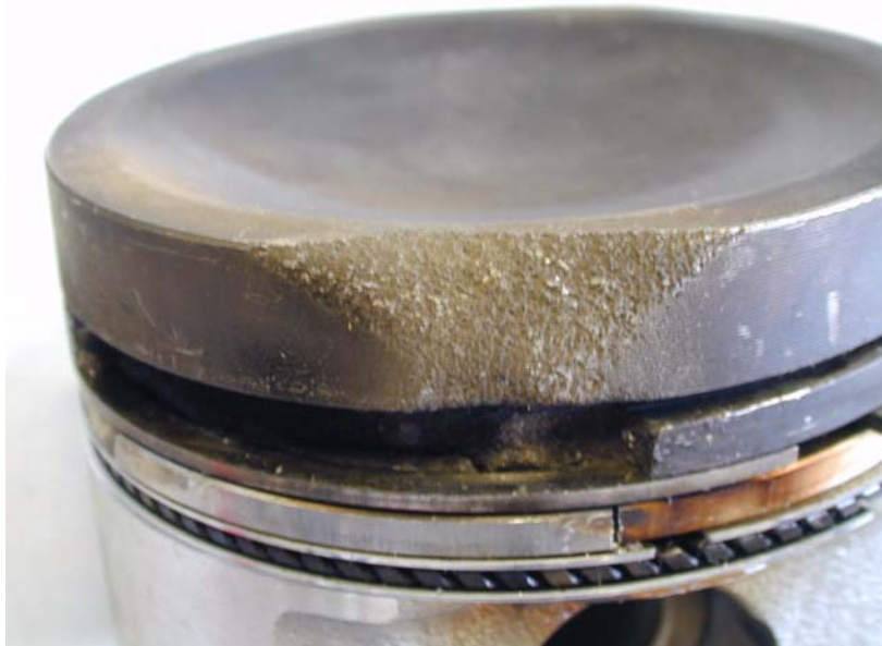
Ignition occurs from hot deposit.
