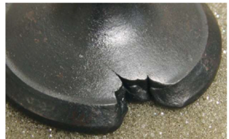
Valve face burning
