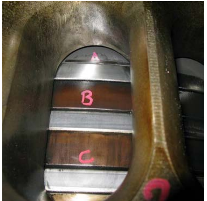
Clean the ring package and mark the piston rings
