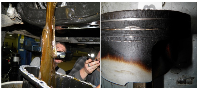
Fig.1. The most severe cases of changes in the motor oil properties [3]: oil transformation into a “rubber-like” mass (left) and complete blocking of the piston rings (right).
